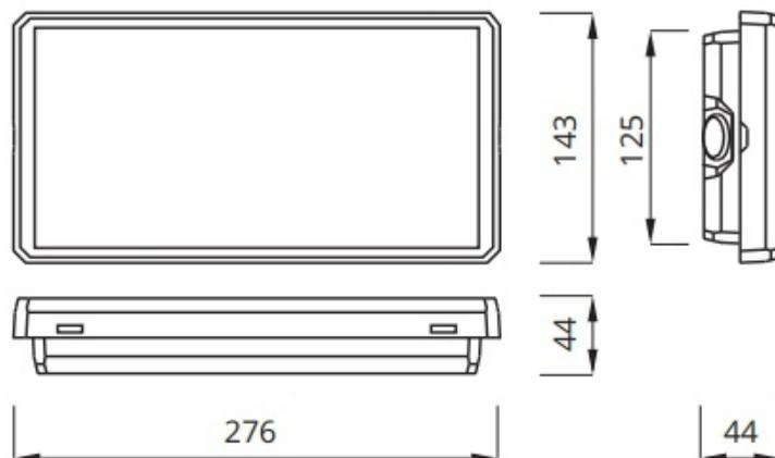
**WYMIARY OTWORU MONTAŻOWEGO (mm):**
